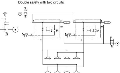
As an alternative to the 2/2 valves 3/2 valves can be used for Rapid Release (RR) due to the Blow Off Valve built into 2BV Ejector
