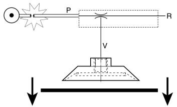
Vacuum is generated when the ejector is supplied with air. If the air supply would be interrupted by e.g., a compressor failure, a malfunctioning valve or a loose connection, the vacuum will not be maintained as atmospheric pressure leaks into the suction cup, causing an unforeseen drop of the object.
