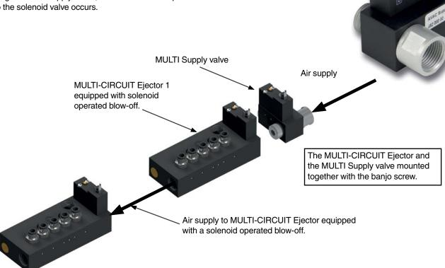
The solenoid operated supply valve can easily be mounted with the banjo screw in the supply port of the ejector. The air flow of the valve is sufficient to supply an number of ejectors in serie and is only intended to be used in combination with solenoid operated blow-off
